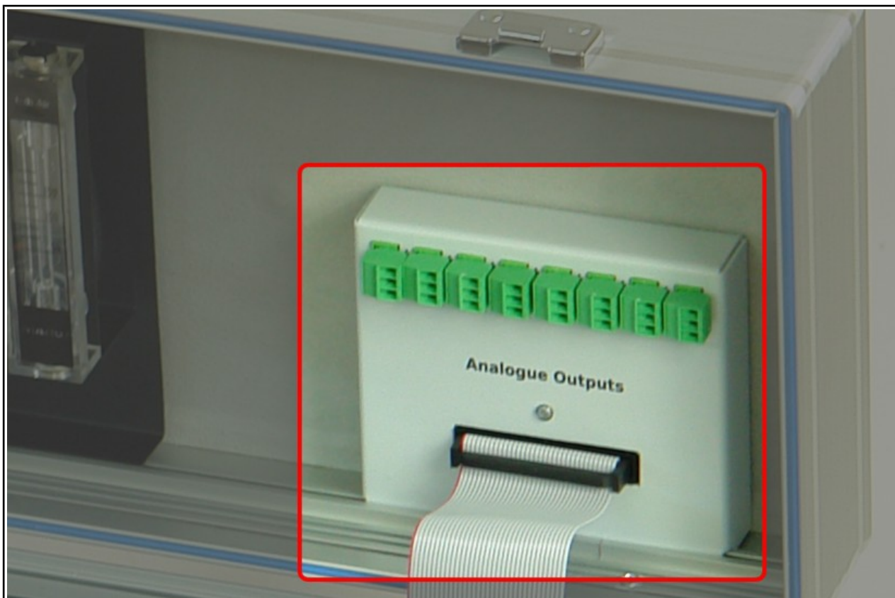
Drawing 2. Localisation of the analogue outputs module in the analysers lid.
